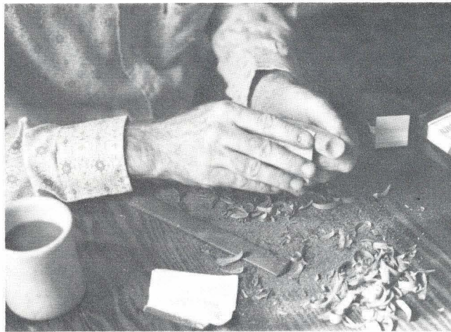
Sand the plug after the shaping is completed. Start with rough sandpaper and finish with fine paper.
