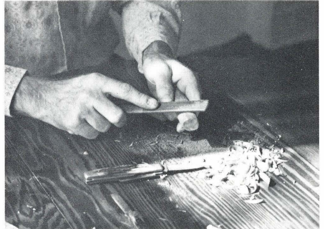
A wood rasp can be used to accomplish final shaping of the plug.
