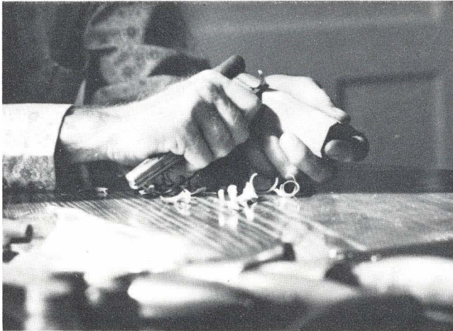
Decide on the style of plug and use a sharp pocket knife to rough cut a block of red cedar.
